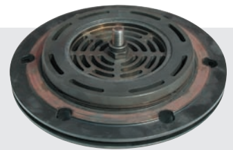
3rd stage air-cooled valve after 2,500 hours
